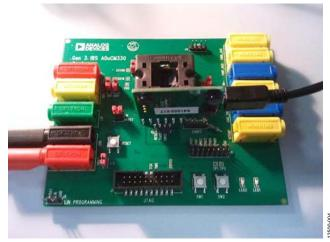
Figure 4. Mini-Link Debugger/Programmer Connection
