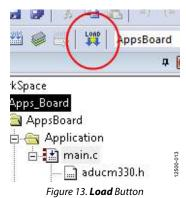
11. When the code is downloaded to the applications board, the two LEDs blink repeatedly.
