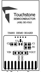
Figure 3. Top Layer Component View
