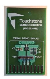
Figure 1. TS6001 Evaluation Board Circuit
