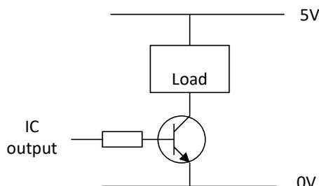
Fig B – Transistor turned off
