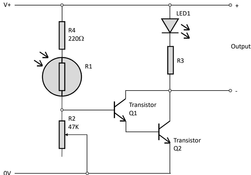
The circuit operation is very simple. When the input to the transistor Q1, which is fed from the connecting point of R1 and R2, is greater than 1.4V, the output is turned on. The voltage at the join of R1 and R2 is determined by the ratio of the two resistors. This is known as potential divider.
