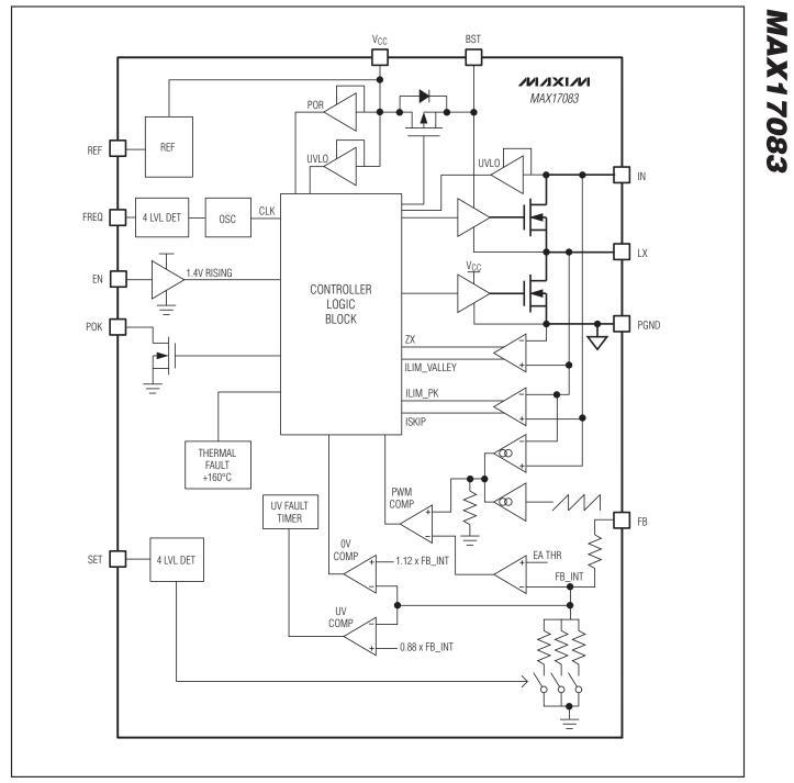
Figure 2. MAX17083 Block Diagram
