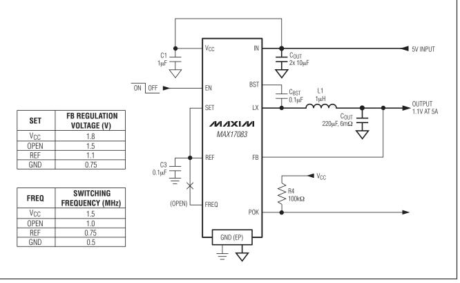
Figure 1. Standard Application Circuit
