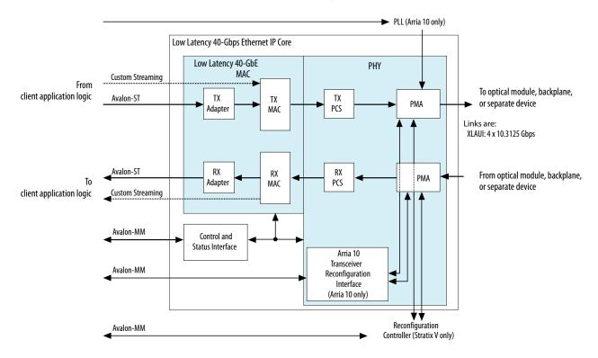
Main blocks, internal connections, and external block requirements.
