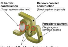
V notch and Double contact constructions
