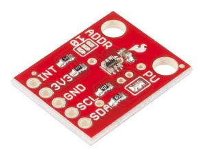
The TSL2561 is an inexpensive, yet sophisticated, light sensor. Unlike simpler sensors, like photoresistors and photodiodes, the TSL2561 incorporates both infrared and visible light sensors to better approximate the response of the human eye. Because the TSL2561 is an integrating sensor (it soaks up light for a predetermined amount of time), it is capable of measuring both very small and very large amounts of light.
