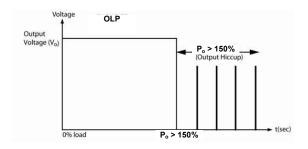
Additionally, if the  $P_{\rm O}$  is < 150% but > 100% for a prolong period of time (depending on the load), the Over Temperature Protection (OTP) will be activated due to high temperature on critical components. The power supply will then go into "Hiccup mode" until power supply cool down.
