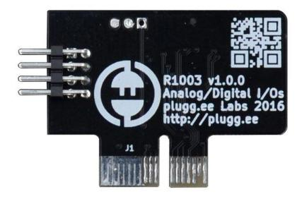
This module connects four microcontroller signals to any external component (such as a thermistor or end-stop switch). It can be used for analog and digital signals.
