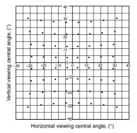
2. Each pixel's viewing angle (half angle) Central 4 pixels (Pixel No. 28, 29, 36, 37) viewing angle (half angle): horizontal direction 7.5° (Typical) vertical direction 8° (Typical)
