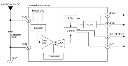
$^{\ast}$  INT terminal 0 normally has same voltage as VDD. When interrupting, same as GND (0V).
