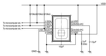
2. In case of setting I<sup>2</sup>C slave address of the sensor 1101001 \* Connect terminal (5) (AD\_SELECT) to VDD.
