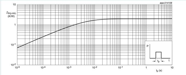
Fig. 7. Transient thermal impedance from junction to mounting base as a function of pulse width
