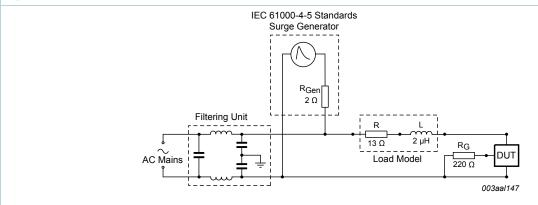
Fig. 6. Test circuit for inductive and resistive loads with conditions equivalent to IEC 61000-4-5
