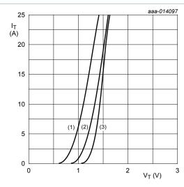
$V_0 = 1.018 \text{ V}; R_s = 0.028 \Omega$
