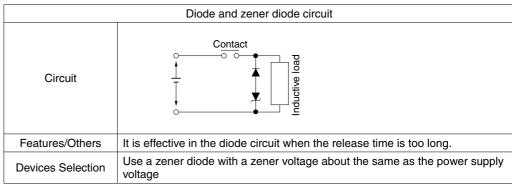
In the actual circuit, it is necessary to mount the protective device (diode etc.) in the immediate vicinity of the load. If it is mounted too far away, the effectiveness of the protective device may diminish. As a guide, the distance should be within 50cm.
