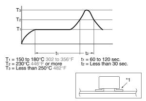
Note: Temperature profile indicates the temperature of the soldered part (\*1) of terminals on the surface of a circuit board. The exterior temperature of a relay may be extremely high depending on the component density on the board or the heating method of the reflow oven or circuit board type. Sufficient verification under actual processing conditions is required. Performance-guaranteed temperature varies by product. Please refer to the relevant product catalog.
