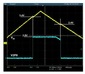
FIGURE 8. THE V2P8 PIN OUTPUT VS THE INPUT VOLTAGE
