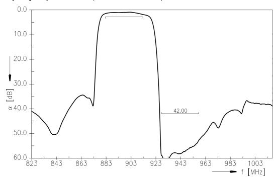
Frequency Response TX-Ant (CW test signal, specification temperature range T=0 °C to +90 °C)
