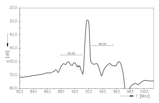
Frequency Responce TX-RX (differential, CW signal, spec temperature range T=0°C to +90°C)
