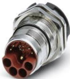
Device connector for rear wall, straight, shielded: yes, Screw locking, M23, No. of pos.: 4+4+4+PE / 3+N+PE, type of contact: Pin, Crimp connection, Flat gasket, Central fastening M26 x 1, Panel thickness min.: 1.5 mm, Panel thickness max.: 5 mm
