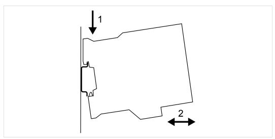
Fig. 3 Mounting on DIN rail
