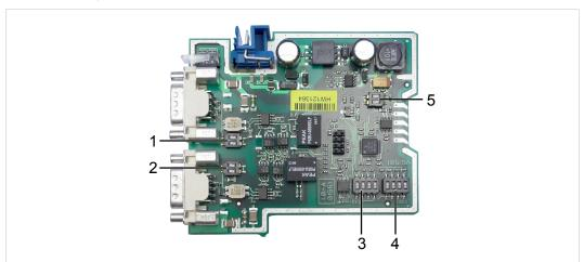
Fig. 2 DIP switches CAN-CR200
