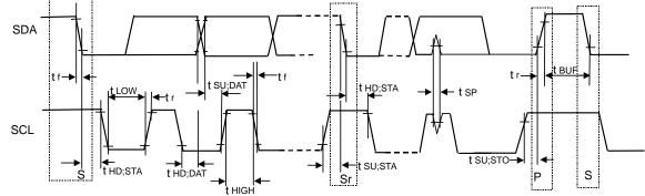
Figure 7. I<sup>2</sup>C timing diagram
