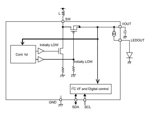
Any I<sup>2</sup>C 'write command' activates the internal blocks of the BD6164GUT, in order to be ready for LED activation. However, if the write command is not immediately followed by a flash or assistant light command, please apply a read command to ensure the IC is going back to low-current standby mode.
