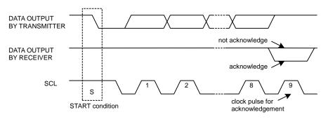
Figure 3. I<sup>2</sup>C Acknowledge waveform
