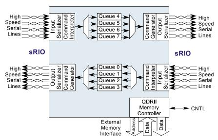
Figure 5. SerB as a FIFO between two FPGAs
