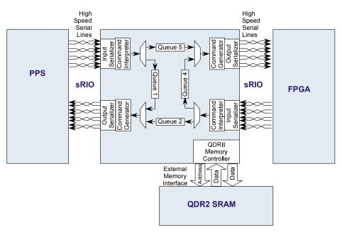
Figure 4. PPS Combined with an FPGA (Distributed)
