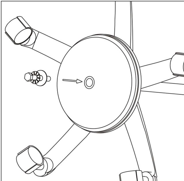
4. Place the weight and the cover under the trolley, see pic. Face the metal cover closest to the trolley.
