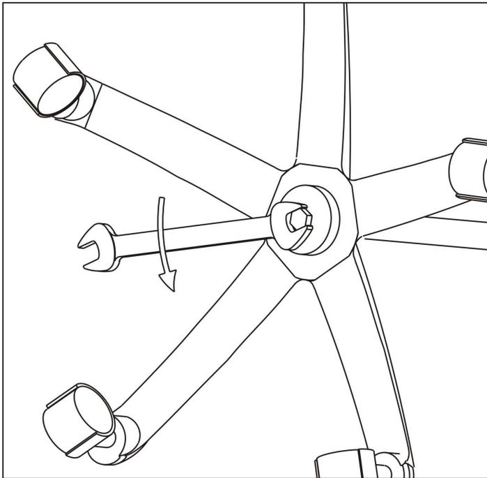
1. Unscrew the bolt underneath the trolley
