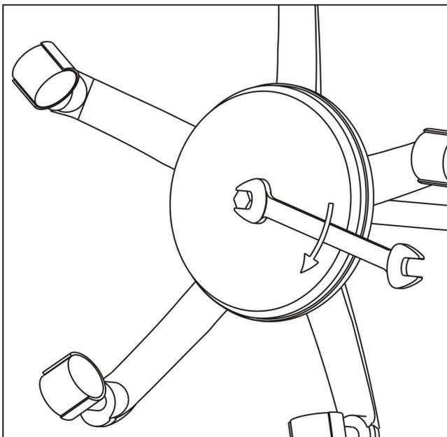
5. Place the bolt with washer through the weight and inside the trolley. Tighten the bolt with a tool, see pic.
