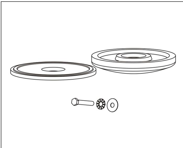
2. The extra weight kit consists of cast iron weight, metal cover and 1 bolt with washer
