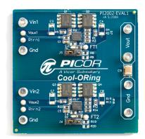
Figure 24: PI2002 Mounted on PI2002-EVAL1
