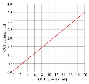
Figure 3: OCT Off time vs. OCT capacitor value
