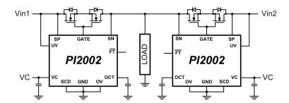
Figure 1a: PI2002 High Side ORing with load disconnect
