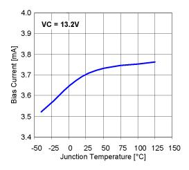
Figure 8: Controller bias current vs. temperature
