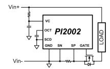
Figure 1b: PI2002 Low Side Disconnect Switch
