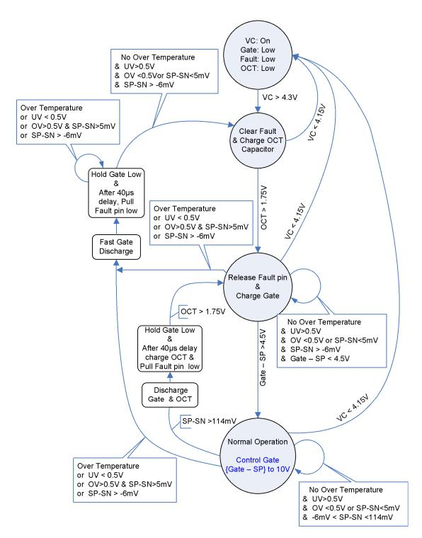
Figure 6: PI2002 State Diagram
