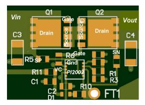
Figure 23: PI2002 and MOSFET layout recommendation
