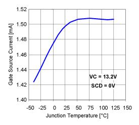
Figure 15: Gate output source current vs. temperature
