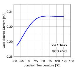
Figure 16: Gate output source current vs. temperature
