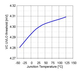
Figure 9: VC UVLO threshold vs. temperature
