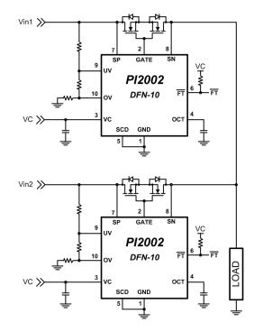
Figure 19: High side Active ORing function.
