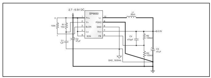
Fig. 24: Application circuit with highlighted power traces.
