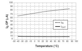
Fig. 13: Quiescent Current vs. Temperature.  $V_{\text{IN}} = 3.6 \text{V, SHDN} = V_{\text{IN}} \text{ (Enabled)}$
