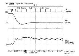
Fig. 18: Dead Short.  $V_{IN}=5.0V$ ,  $I_{LIM}$  tied to GND. Start  $I_{OUT}=37$ mA,  $V_{OUT}=3.3V$ . Finish  $I_{OUT}=500$ mA,  $V_{OUT}=20$ mV.
