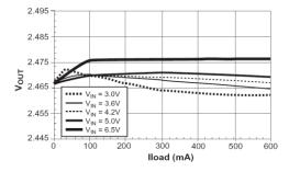
Fig. 8: Line/Load Rejection,  $V_{\text{OUT}}$  = 2.5V, L1 = 22 $\mu$ H (Sumida CDRH6D28),  $I_{\text{LIM}}$  =  $V_{\text{IN}}$
