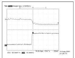
Fig. 20  $V_{OUT}$  transient response from 50mA to 500mA load step. CH1-  $V_{OUT}$ , CH4 -  $I_{LOAD}$
