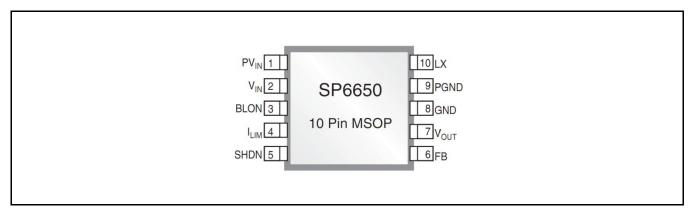
Fig. 3: SP6650 Pin Assignment
