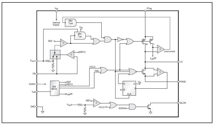
Fig. 2: SP6650 Block Diagram
