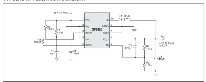
Fig. 1: SP6650 Application Diagram
