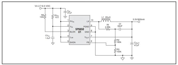
Fig. 19: Additional Application Circuit with Low Output Ripple
