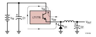
Figure 3. High Speed Current Switching Paths
