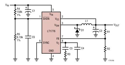
Figure 5. User Programmable Undervoltage Lockout
