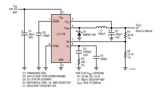
Figure 4a. Minimum Component Count Application
