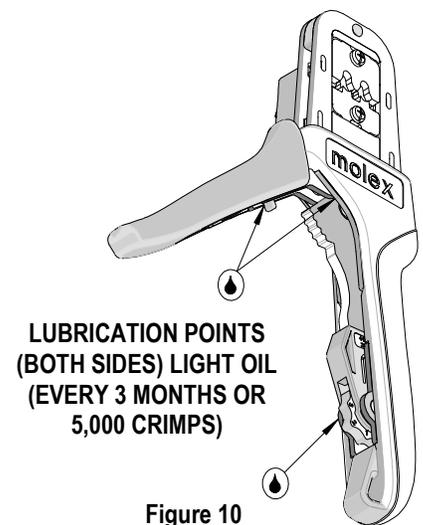
3. Make certain all pins; pivot points and bearing surfaces are protected with a thin coat of high quality machine oil. Do not oil excessively. The tool was engineered for durability but like any other equipment it needs cleaning and lubrication for a maximum service life of trouble free crimping. Light oil (such as 30 weight automotive oil) used at the oil points, every 5,000 crimps or 3 months, will significantly enhance the tool life.
