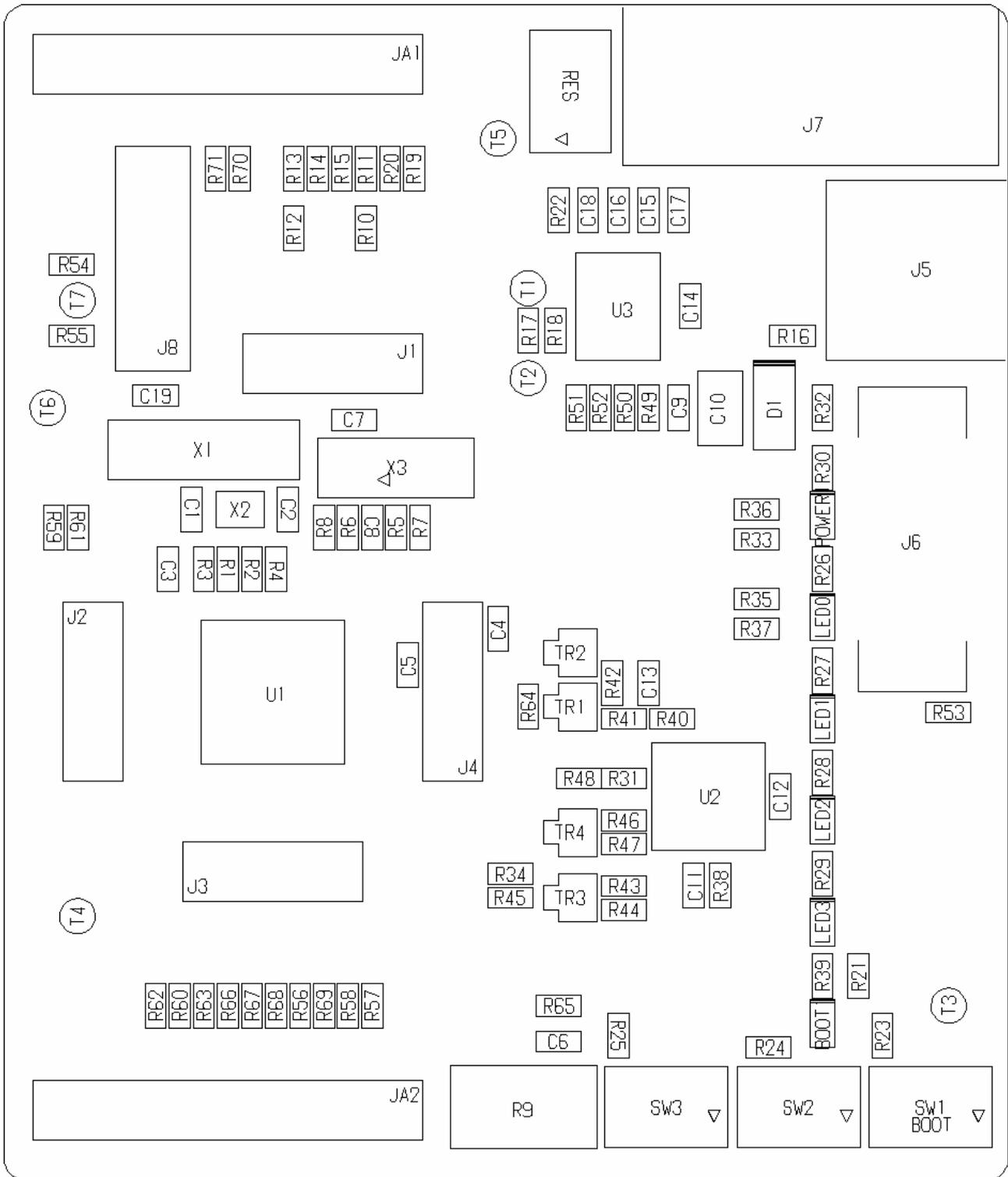
Figure 11-1: Component Placement
