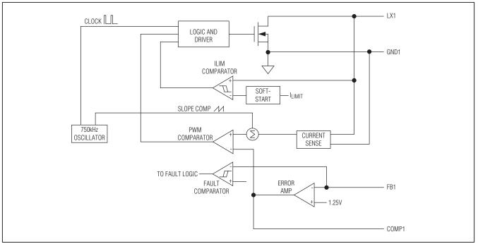
Figure 3. Step-Up Regulator Block Diagram
