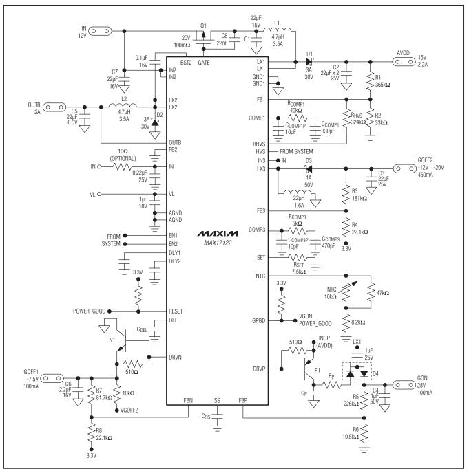
Figure 1. Typical Operating Circuit
