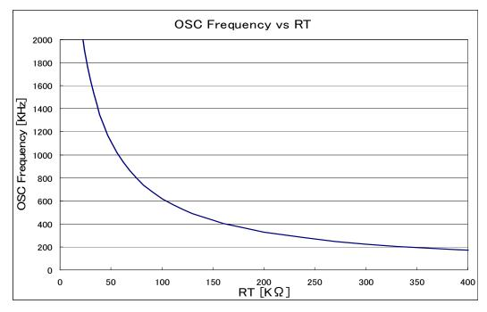
Figure : switching frequency vs external resistance
