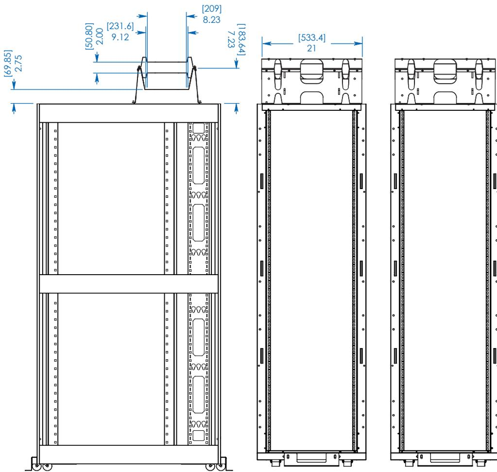
OPTIONAL SRCABLETRAY AND SRCABLETRAYEXP CABLE MANAGEMENT ACCESSORIES SHOWN (MOUNTING POSITION ADJUSTS TO ACCOMMODATE A WIDE RANGE OF APPLICATIONS)
