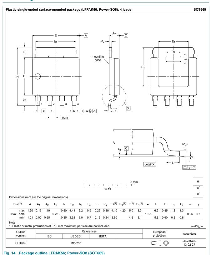
40 V, 10 A NPN high power bipolar transistor
