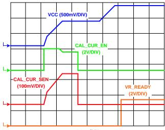
4.0ms/DIV FIGURE 3. SOFT-START/CALIBRATION SEQUENCE (3-PHASE)
