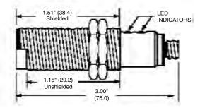
Note: Mounting hole dimensions are in mm and (inches).
