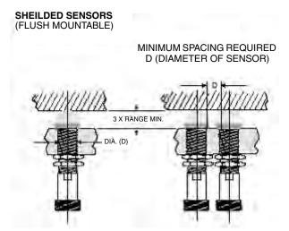
SENSORS MUST BE MOUNTED SUCH THAT SURROUNDING METAL IS NOT IN THE SENSING AREA.
