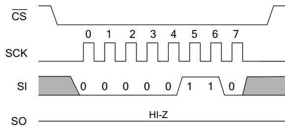
**WRDI - Reset Write Enable Latch**
