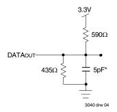
Figure 1. AC Output Test Load
