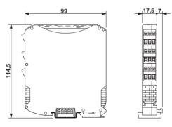
Figure 3 Dimensions (in mm)
