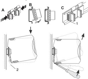
Figure 4 Assembly and removal
