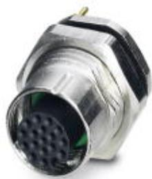
Sensor/actuator flush-type connector, socket, 17-pos., M12 SPEEDCON, shielded, A-coded, rear/screw mounting with Pg9 thread, with straight solder pins
