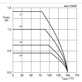
FR4 PCB, mounting pad for anode and cathode 1 cm<sup>2</sup> each
