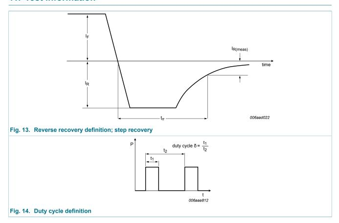
The current ratings for the typical waveforms are calculated according to the equations:  $I_{F(AV)} = I_M \times \delta$  with  $I_M$  defined as peak current,  $I_{RMS} = I_{F(AV)}$  at DC, and  $I_{RMS} = I_M \times \sqrt{\delta}$  with  $I_{RMS}$  defined as RMS current.
