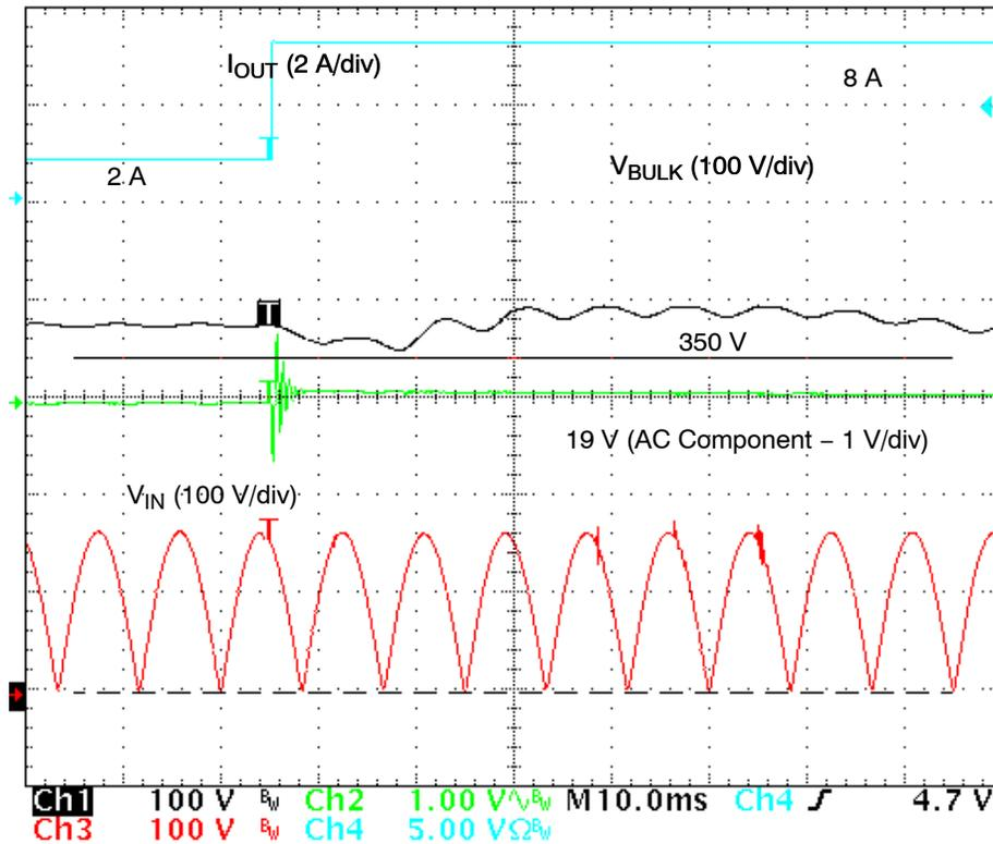
Figure 15. Abrupt Load Increase at 120 Vrms
