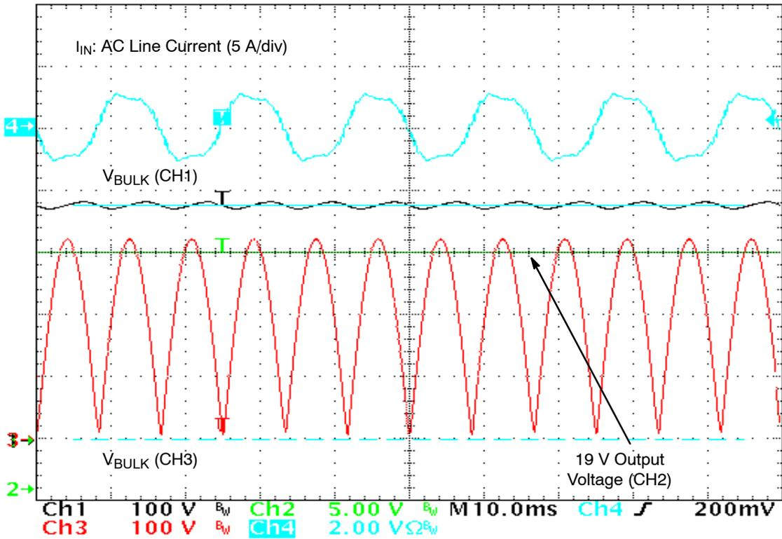
$V_{IN,RMS} = 230$  V,  $P_{in} = 177$  W,  $I_{OUT} = 8$  A, PF = 0.976, THD = 17%
