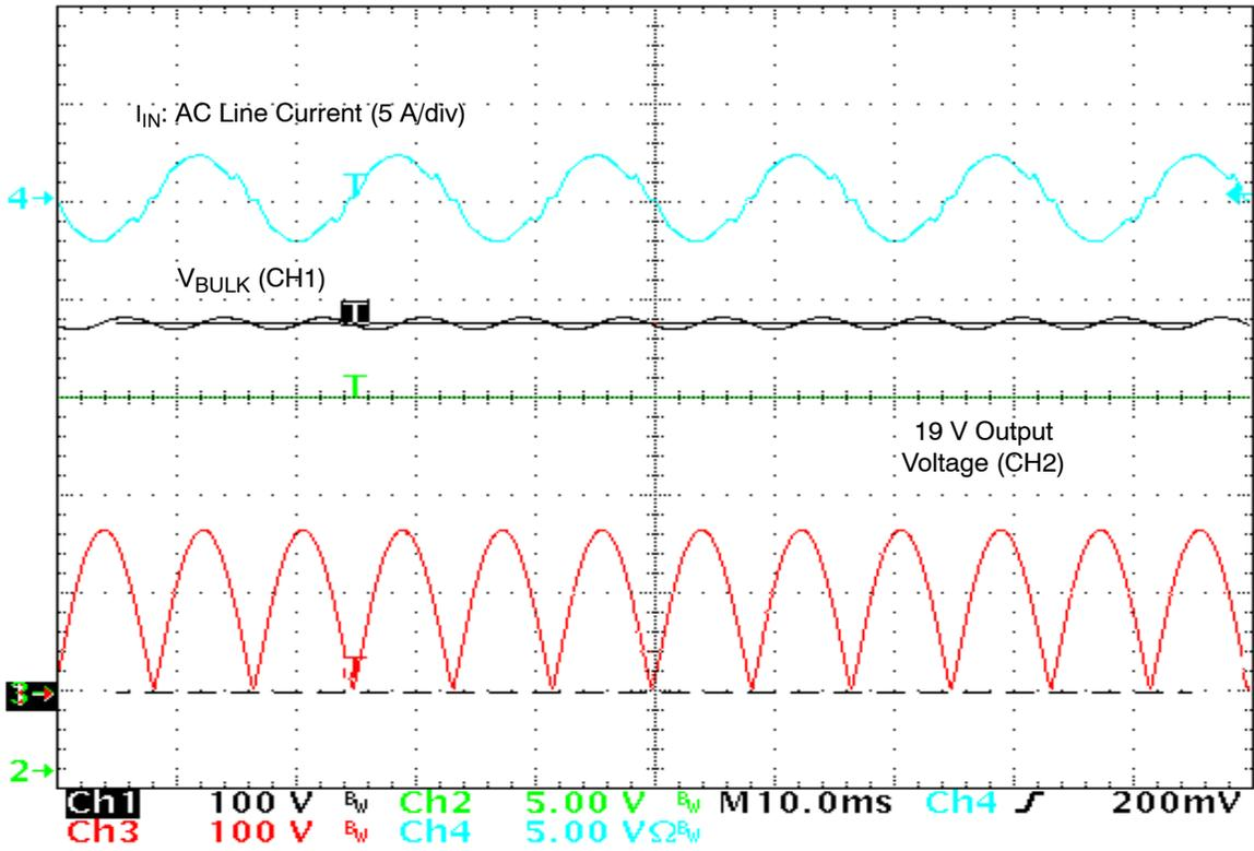
$V_{IN,RMS} = 120$  V,  $P_{in} = 183$  W,  $I_{OUT} = 8$  A, PF = 0.992, THD = 10%
