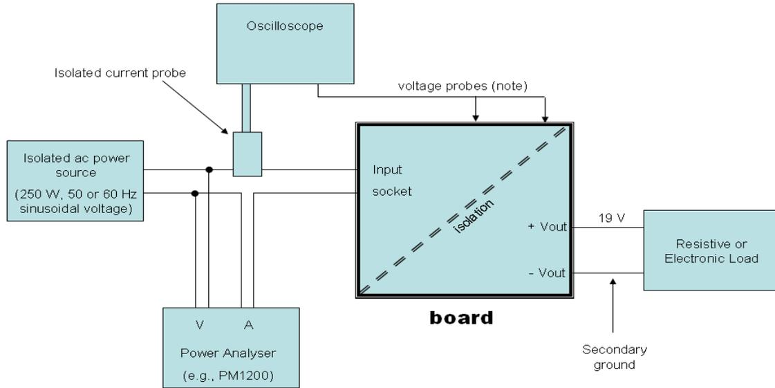
Note: use as many voltage probes as needed to display the waveforms you want to observe. Please note that high-voltage ones may be necessary since the voltage across some parts of the board can be as high as 500 V (that across the power MOSFETs of both stages for instance).
