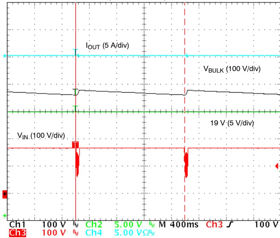
Figure 17. Skip Mode Operation of the PFC Stage at 120 Vrms, No Load.
