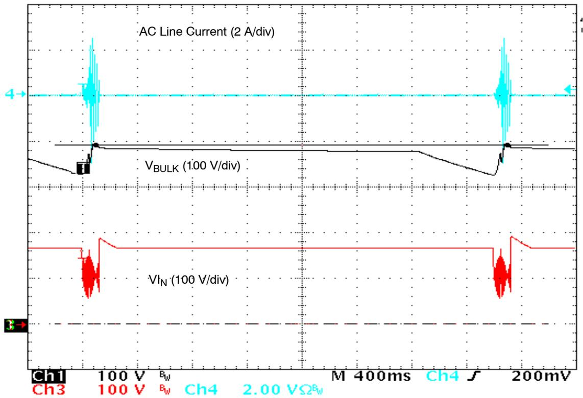
Figure 11. The Circuit Enters a Safe Low Duty-Cycle Hiccup Mode if the 19 V Output is Short Circuited (Test Made at 120 V<sub>RMS</sub>)
