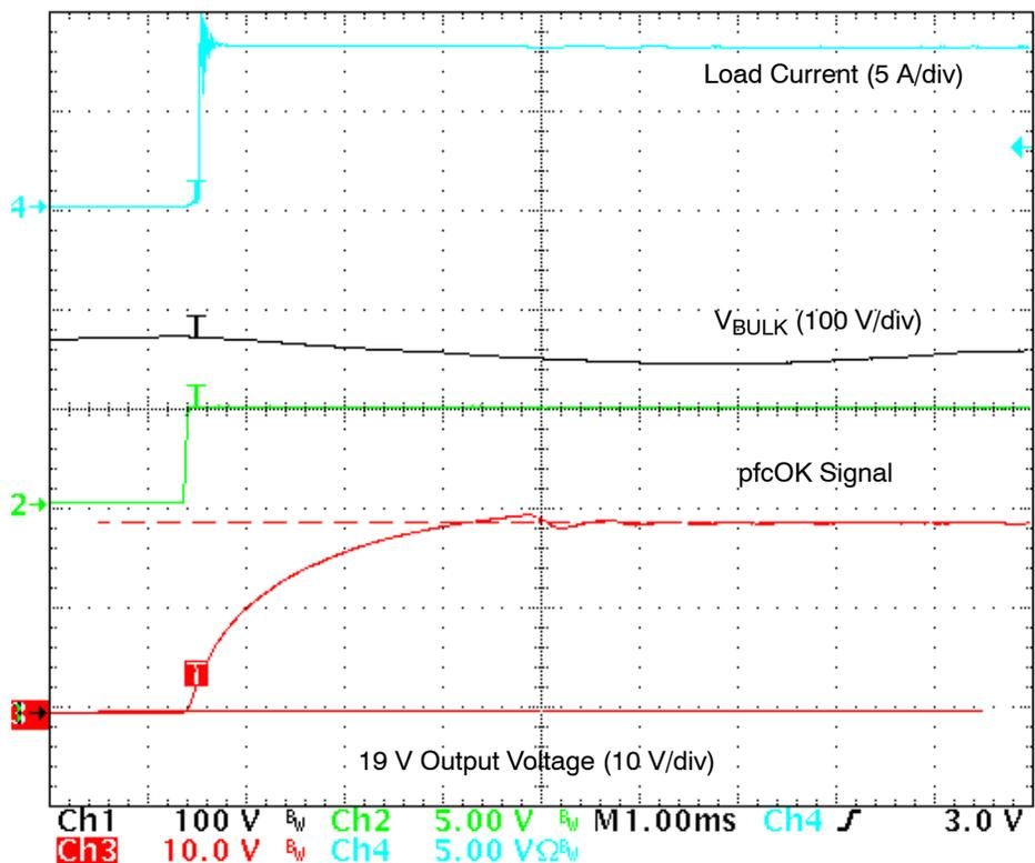
Figure 10. Startup Phase at 120 Vrms
