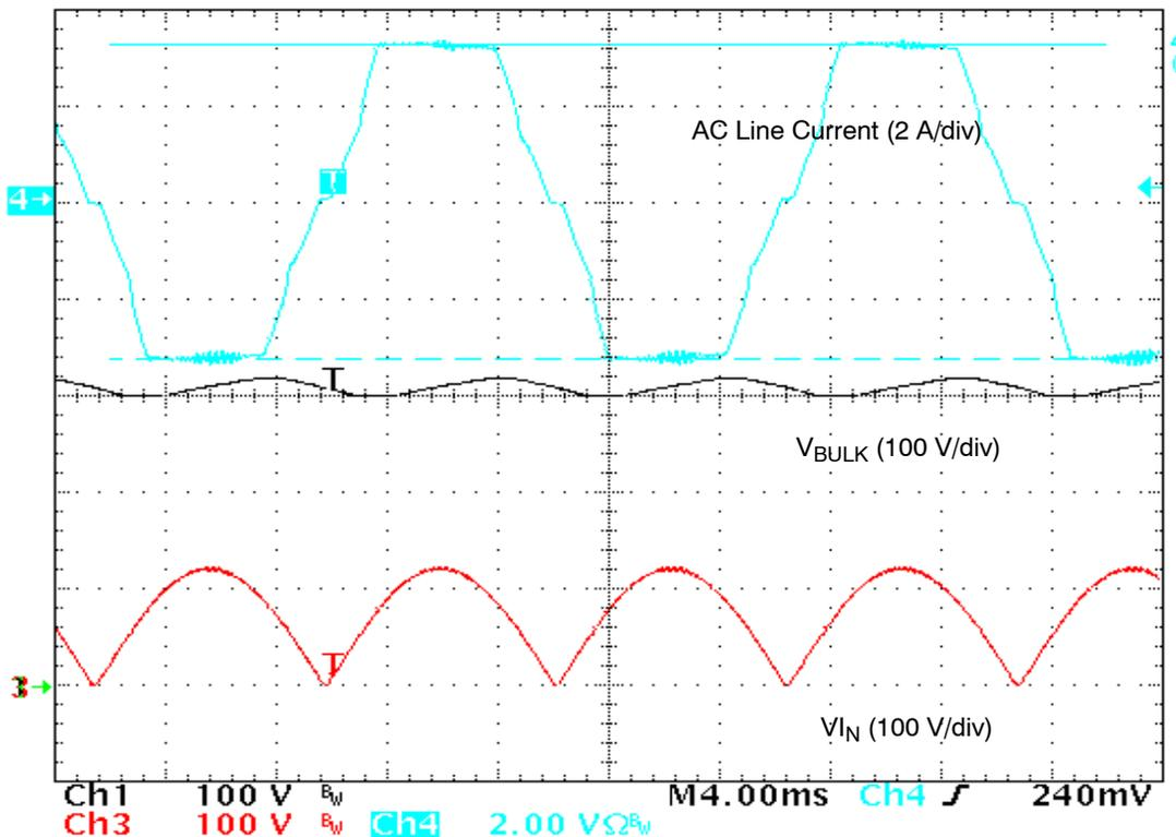
**Figure 14. Action of the Overcurrent Limitation**
