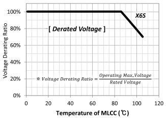
This product ,which guarantees High Temperature Reliability Test with 100% of rated voltage at the maximum temperature, is recommended to be used in the circuit with derated voltage compared to the rated voltage of the capacitor for long lifetime.
