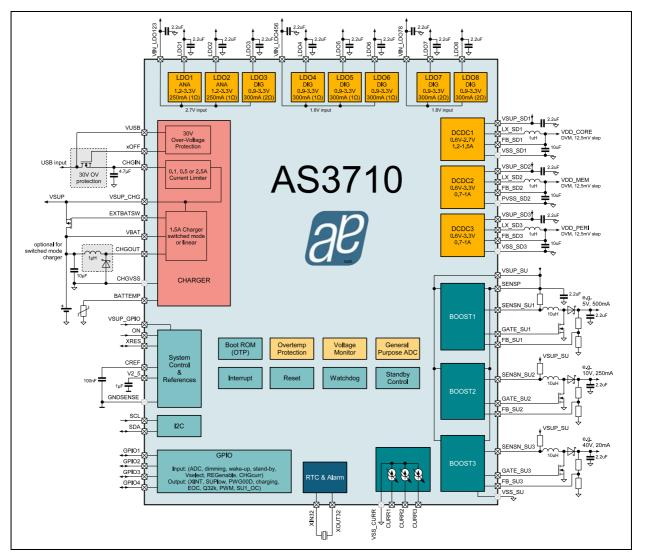
Figure 1. AS3710 Block Diagram
