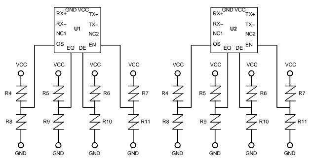
Figure 4. Resistor Pads to Set DC Control Pins
