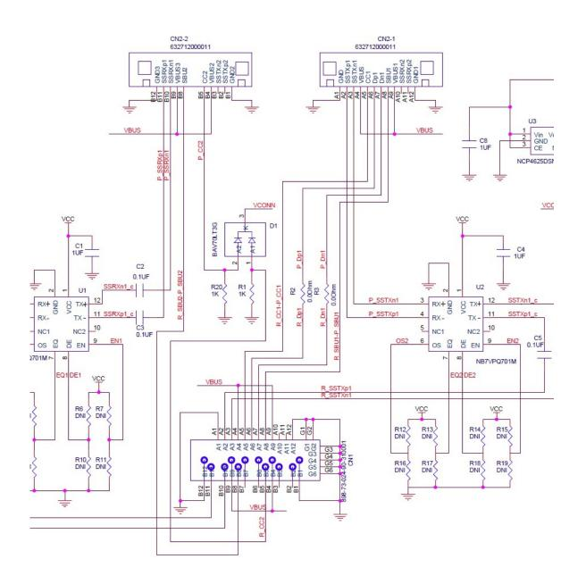
Figure 7. NB7VPQ701MMEVK Schematic
