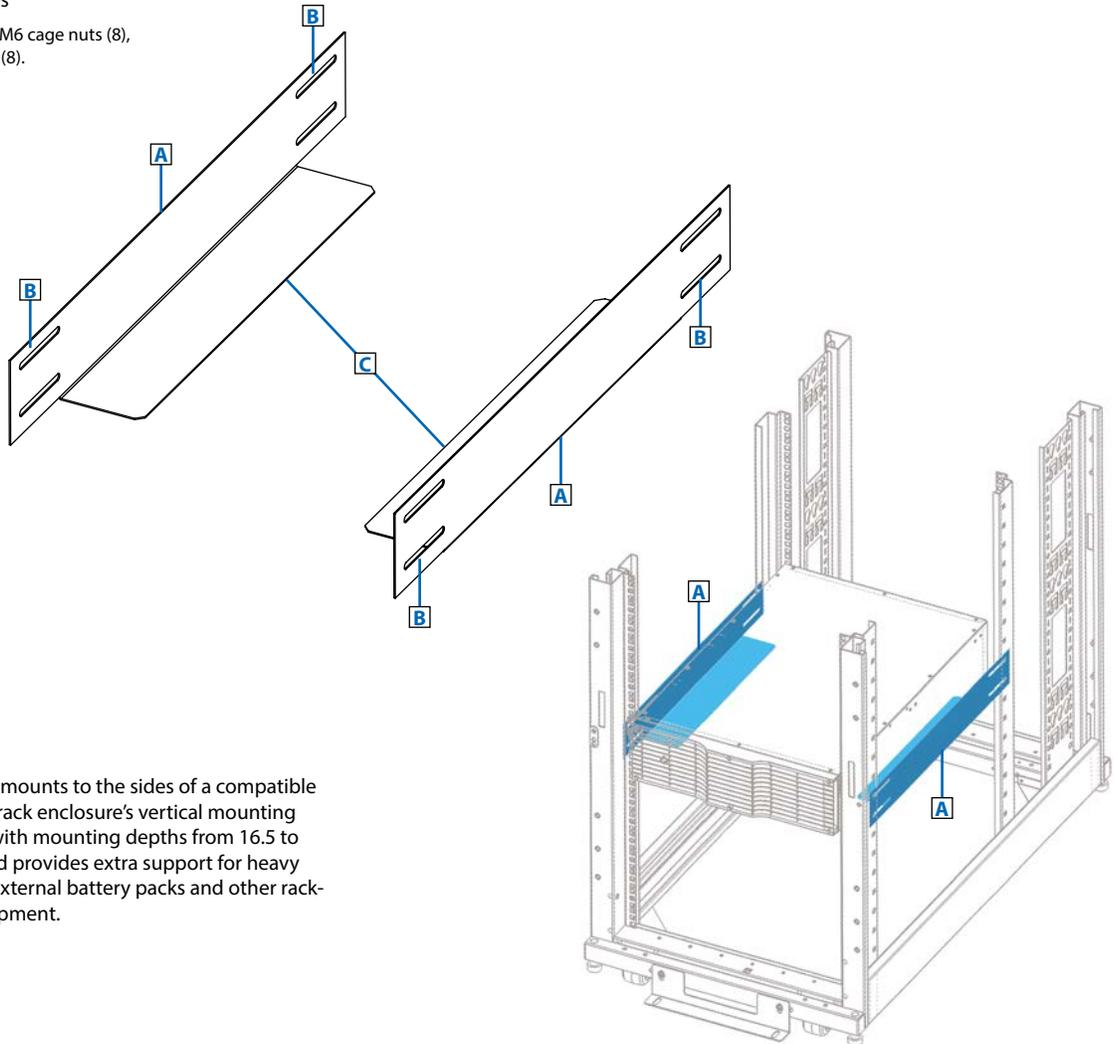
4POSTRAILSM mounts to the sides of a compatible 4-post rack or rack enclosure's vertical mounting rails. It works with mounting depths from 16.5 to 21.5 inches and provides extra support for heavy UPS systems, external battery packs and other rack-mounted equipment.
