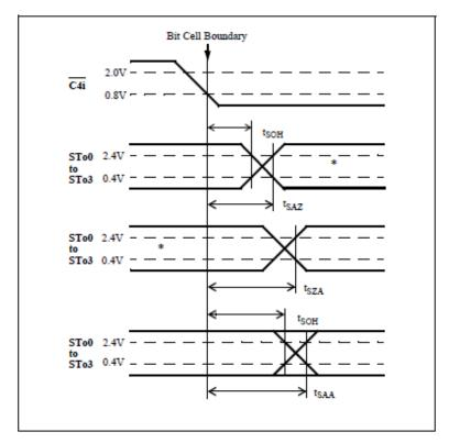
Figure 14 - Serial Outputs and External Control
