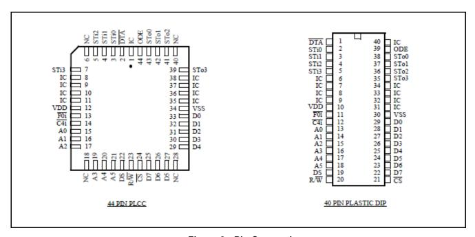
Figure 2 - Pin Connections
