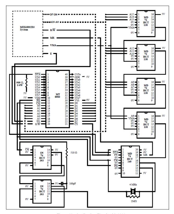
Figure 10 - Application Circuit with 6802
