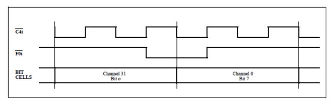
Figure 12 - Frame Alignment
