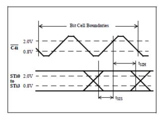
Figure 16 - Serial Inputs
