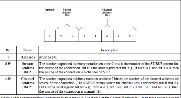
\*If bit 2 of the corresponding Connection High location is 1 or if bit 6 of the Control Register is 1, then these entire 8 bits are output on the channel and stream associated with this location. Otherwise, the bits are used as indicated to define the source of the connection which is output on the channel and stream associated with this location.
