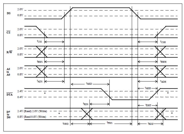
Figure 17 - Processor Bus
