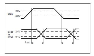
Figure 15 - Output Driver Enable
