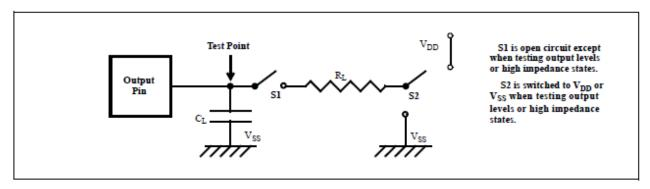
Figure 11 - Output Test Load
