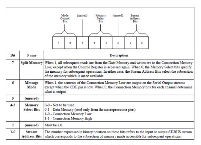
Figure 4 - Control Register Bits
