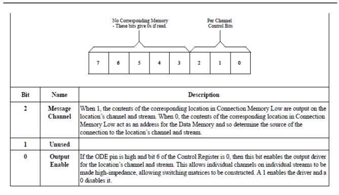
Figure 5 - Connection Memory High Bits
