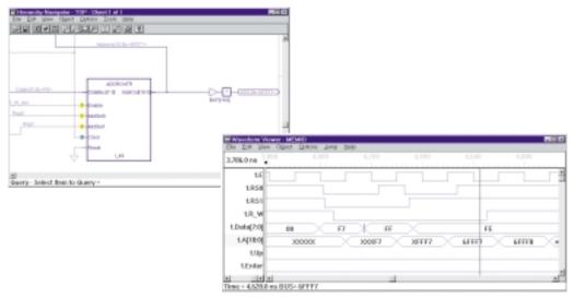
Note: Cross-probing between the schematic and waveform viewer ties simulation results directly back to the source for faster and easier interpretation. Results update each time you single-step the simulator.
