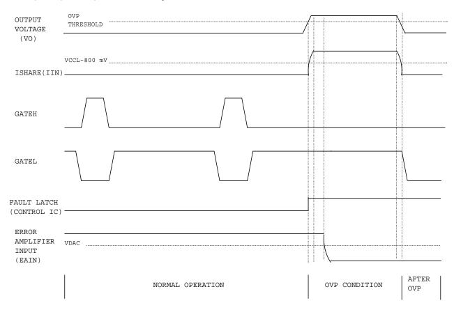
Figure 6 - Over-voltage protection waveforms
