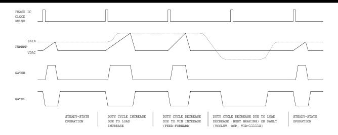
Figure 3 PWM Operating Waveforms
