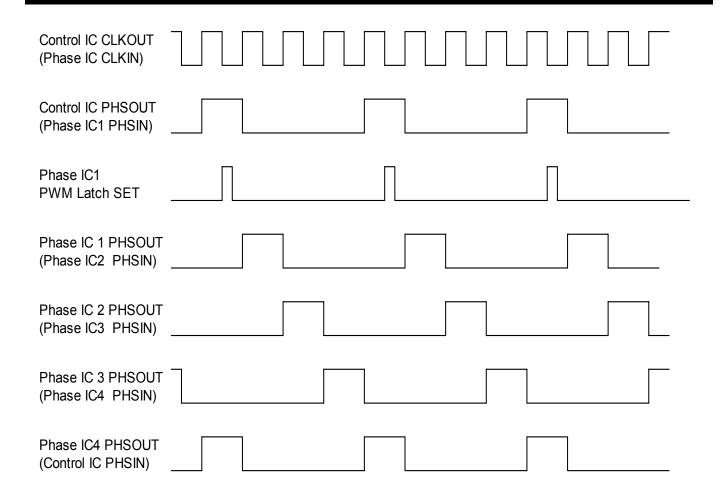
Figure 2 Four Phase Oscillator Waveforms
