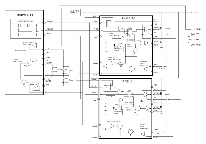
Figure 1 PWM Block Diagram
