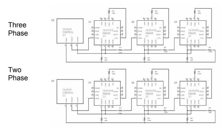
Figure 8 - Optional Phase application circuit
