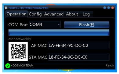
Congratulations, you've loaded the MicroPython firmware on the ESP8266! In the future if you'd like to load the firmware again you can repeat the process above to put the ESP8266 into programming mode and run nodemcu-flasher to upload code.
