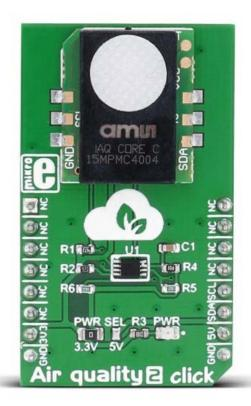
**Air quality 2 click** carries the iAQ-Core Indoor Air Quality sensor that measures VOC (volatile organic compounds) levels and provides CO2 equivalent and TVOC (total volatile organic compounds) equivalent predictions. The click is designed to run on either 3.3V or 5V power supply. It communicates with the target MCU over I2C.
