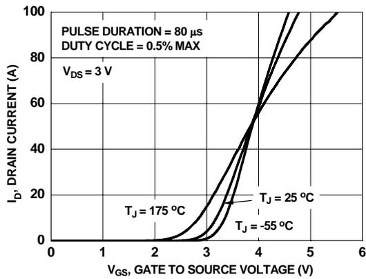
**Figure 5. Transfer Characteristics**
