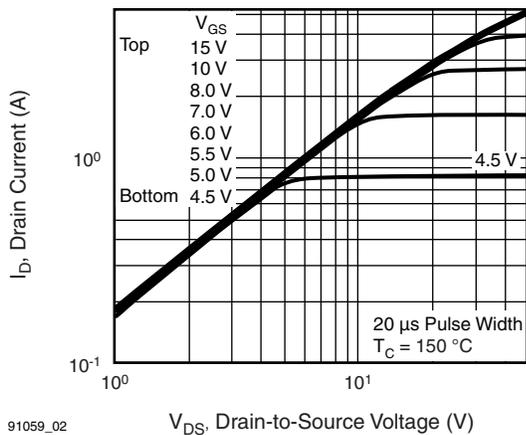
**Fig. 2 - Typical Output Characteristics,  $T_C = 150\text{ }^\circ\text{C}$**
