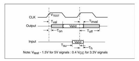
Figure 16-1 PCI Signal Timing Measurement Conditions
