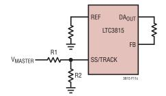
Figure 13c. Slave IC Circuit for Coincident Tracking and  $V_{MASTER} \geq V_{SLAVE}$
