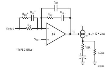
Figure 9. PSPICE Model of a LTC3815 Current Mode Regulator
