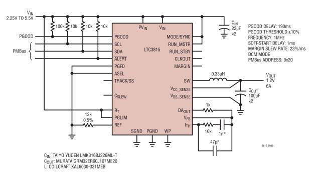
1.2V/6A 1MHz Buck Regulator with Minimum External Components
