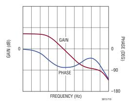
Figure 10. Transfer Function of Buck Modulator
