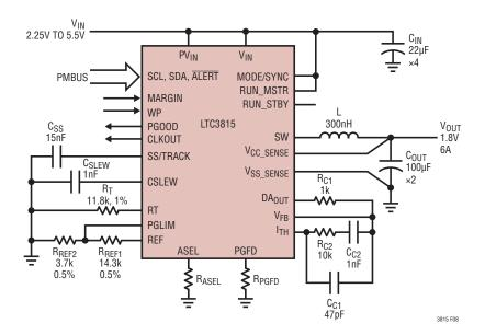
Figure 8. 1.8V, 6A Step-Down Regulator
