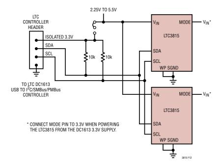
Figure 14. LTC Controller Connection
