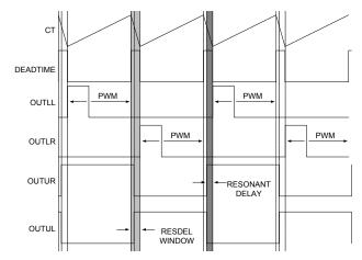
FIGURE 12. BRIDGE DRIVE SIGNAL TIMING
