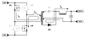
FIGURE 14. UL - LR POWER TRANSFER CYCLE
