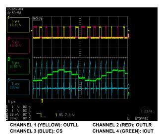
FIGURE 6. DYNAMIC BEHAVIOR OF CS vs IOUT
