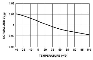
FIGURE 1. REFERENCE VOLTAGE vs TEMPERATURE
