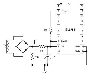
FIGURE 10. ADDING SLOPE COMPENSATION
