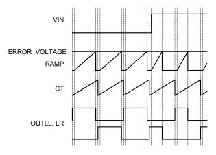
FIGURE 8. VOLTAGE FEED FORWARD BEHAVIOR
