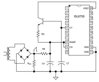
FIGURE 11. ADDING SLOPE COMPENSATION USING CT
