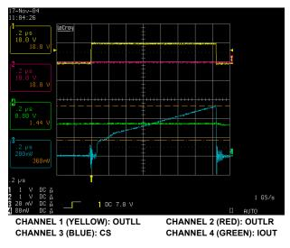
FIGURE 5. CS INPUT vs IOUT
